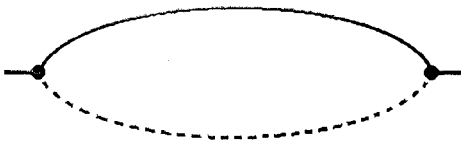
FIG. 2. One-loop correction to the thermal conductivity. The three-point vertices in the diagram are generated by the convective term in the heat transport equation [Eq. (A8b)] and the term (1/\rho)(\delta F/\delta \epsilon)\nabla \epsilon in Eq. (A8c).
